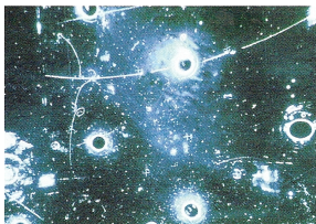
Fig 3. A leptonic weak neutral current event in which the neutrino has scattered off an electron in the heavy liquid by exchanging the Z boson.
